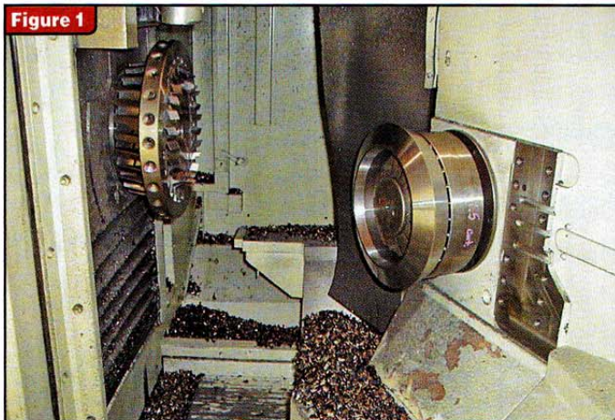
Figure 1 A forged blank is about to be machined with the two-cut process.
