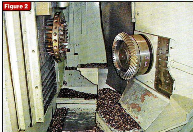
Figure 2 A ring gear finished with the two-cut dry-machining process
