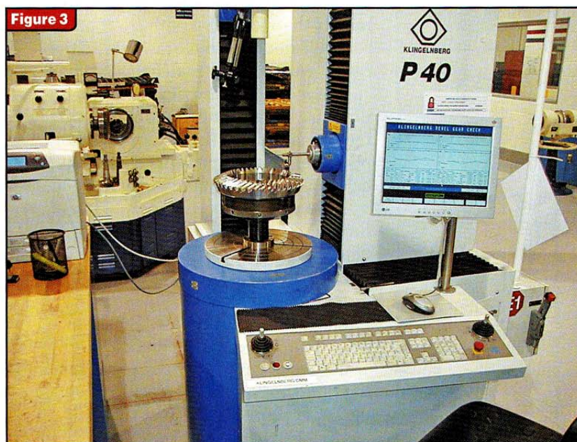
Figure 3 A finished ring gear is measured on a computer-controlled coordinate-measuring machine to check adherence to specifications.
