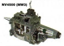
NV4500 – 5-speed manual rearwheel-drive transmission, cast-iron case
