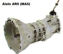
Aisin AR5 – 5-speed rear-wheel-drive manual transmission, over-drive 5th, similar in design to AX15
