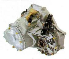
Saab F23 – 5-speed manual front-wheel-drive transaxle, also called MU3 in the service manual
