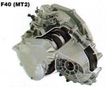
Opel F40 – 6-speed manual front-wheel-drive transaxle
