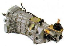
Tremec T56 – 6-speed rearwheel-drive manual transmission, 5th and 6th overdriven
