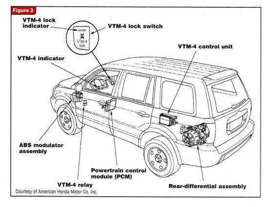
permit the codes to be displayed on the VTM-4 control units as sequenced light blinks. There are 25 possible codes, which we have listed in Figure 4.
