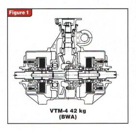
The differential is necessary because the outside wheel on an axle has to cover more distance in a turn than the inside wheel. This means that the outboard wheels must rotate faster than the inboard wheels; hence, the "differential" in wheel speed.
