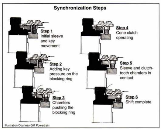
The clutch then is engaged and the throttle is "blipped" to raise the engine speed several thousand rpm higher. The driver then depresses the clutch again and selects the speed gear desired by feel as the engine speed starts to drop and the shaft speeds equalize. The synchronizer accomplishes this without all the fancy footwork.
