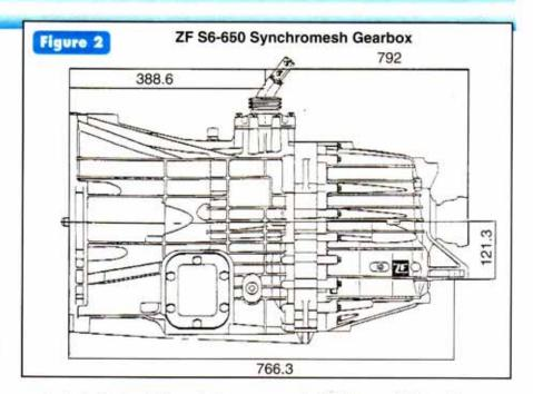
geartrain is designed for quiet operation. The case is aluminum with an integral bellhousing, a center support and an extension housing. The unit uses 5.5 liters of synthetic Mercon ATF and is equipped with an internal pump for pressurized lubrication and an external cooler to keep the internal continues next page
