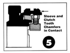
ring relaxes and lines up with the slider, permitting the completion of a smooth, clash-free shift. The unit should then remain in gear no matter what changes are made in the throttle opening. Any wear in these components, excess end play or damaged parts will prevent this sequence from happening. As you can see, understanding the theory is the only way you can evaluate all the components properly before making the repair.
